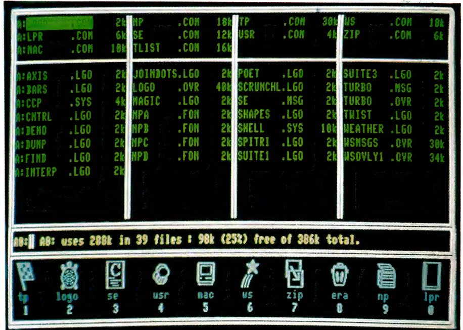
Figure 1. Dealwriter entirely does away with the standard keyboard – every facet of the package can be operated by switches, which can vary in number from nine (as can be seen across the bottom of the screen) down to just one.
