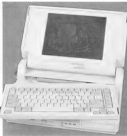
The Compaq SLT 286 is a masterpiece of packaging, with a fast 80286 and a VGA display (we still can't believe how small it is).
